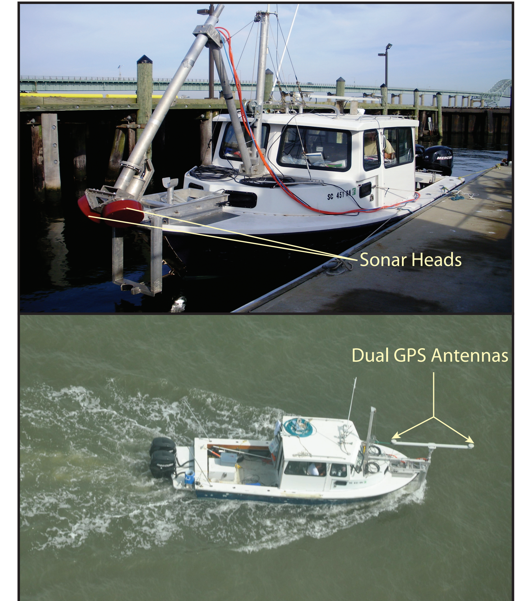
Coastal Carolina University's Privateer with a bow-mounted Kongsberg EM3002d dual-head shallow water multibeam bathymetry system.
