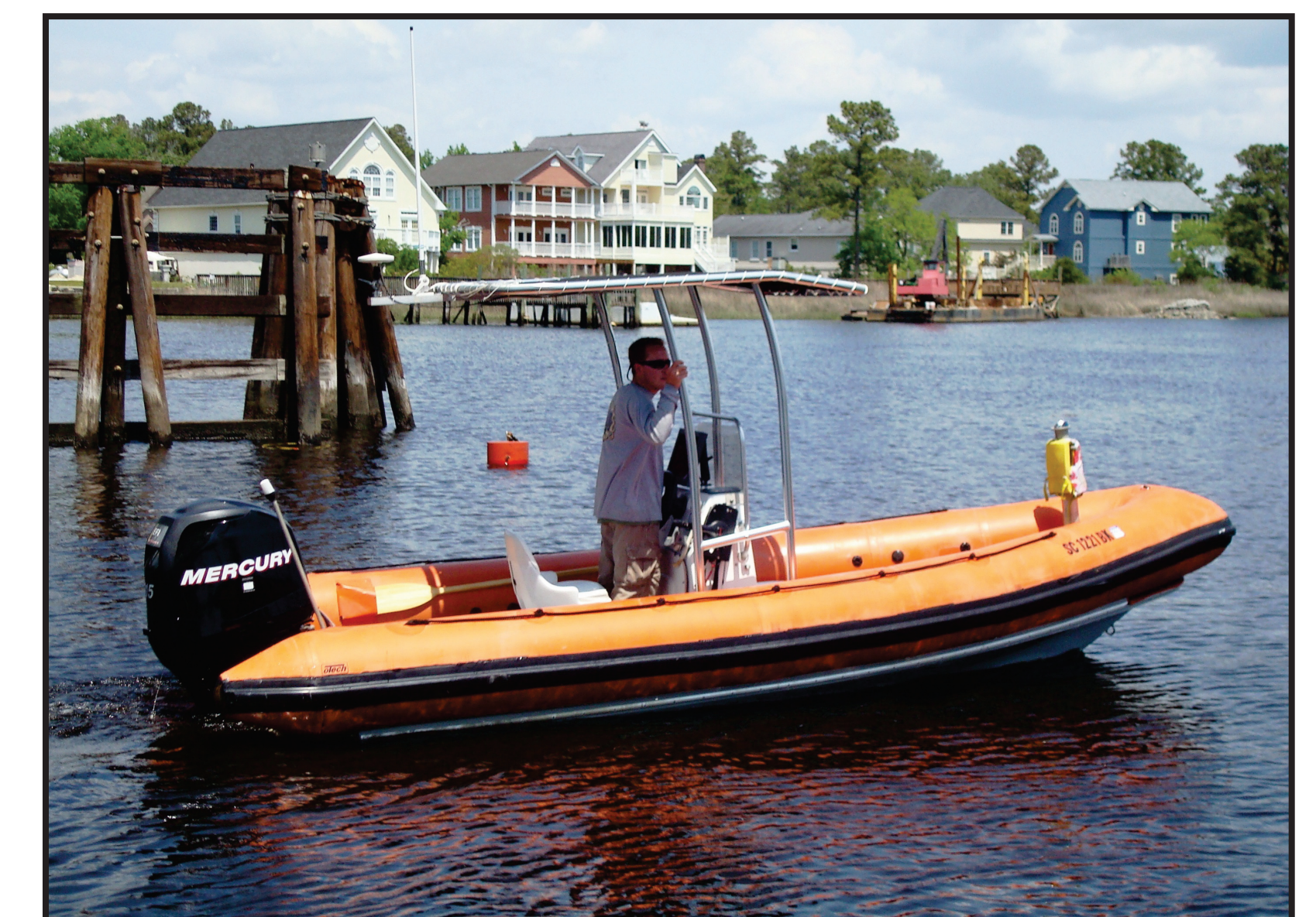
Coastal Carolina University's BERM boat with a single-beam echosounder for shallow water bathymetry.
