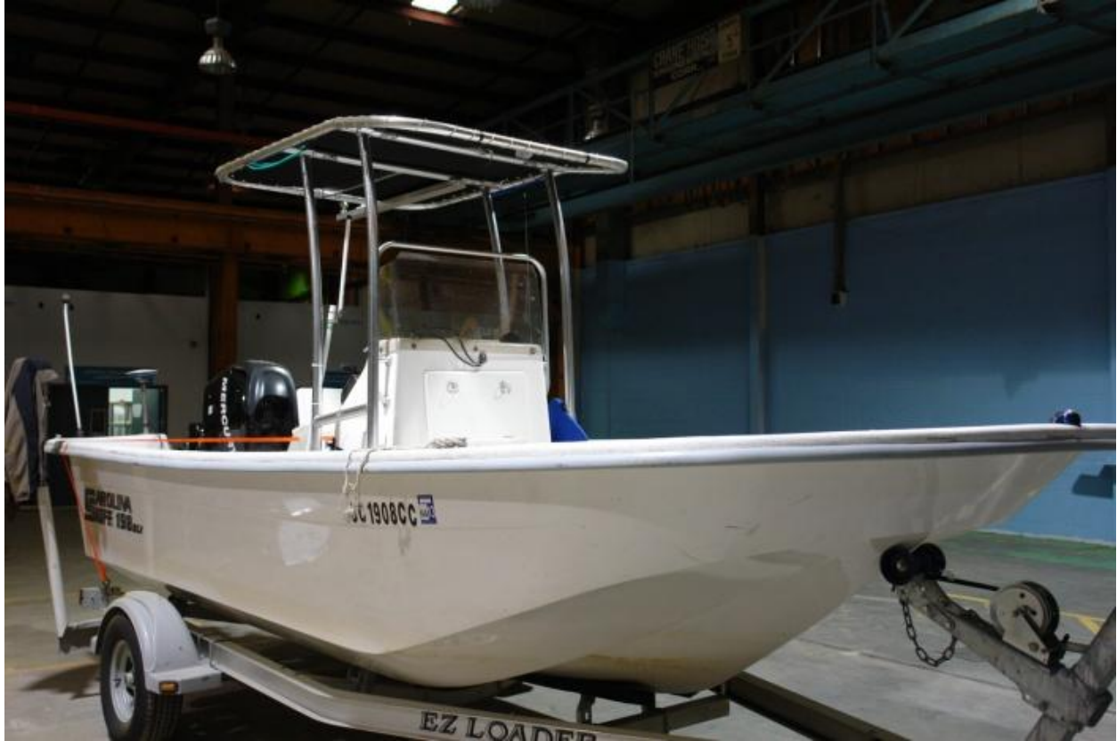
Figure 6. The single beam data acquisition boat, a 20 ft. Carolina Skiff.
