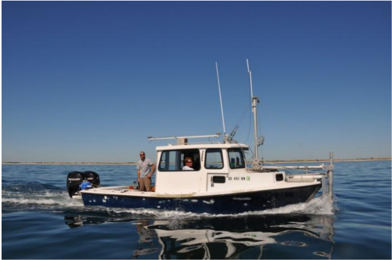
Figure 4. The multibeam data acquisition boat, a 24 ft. Privateer.
